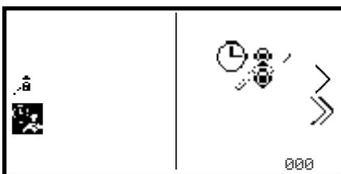
This stage allows an air gap to be added to the calibration sequence. If an air gap is not required press the key below the **000** icon to set the air gap to zero. If a previously programmed air gap is to be used press the key adjacent to the **double greater than** icon to skip this stage and retain the current air gap time.
