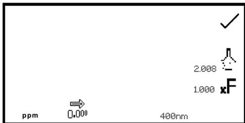
The settings menu is accessed through the expanded operating menu by pressing the key adjacent to the **settings** icon. In the settings menu press the key below the **wavelength** icon.
