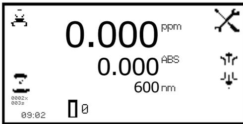
The **autolog** function enables repeat measurements of the same sample to be performed with a set time period between each measurement. This produces a batch of results for the same sample. The autolog function also enables the results to be autologged to different destinations. The autolog menu is accessed from the utility toolbar in the expanded operating menu by pressing the key adjacent to the **autolog** icon.
