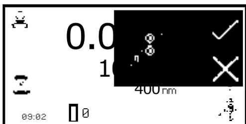
Confirmation will be needed to start the sipper pump. Press the key adjacent to the **tick** icon to confirm and start the sipper pump. Press the key adjacent to the **cross** icon to cancel and return to the expanded operating menu.
