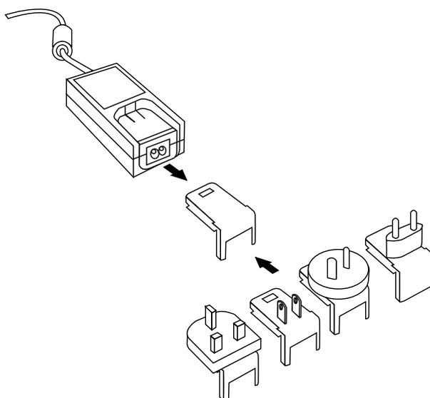
**Fig 2.2.1 – Power supply unit with various plugs**
