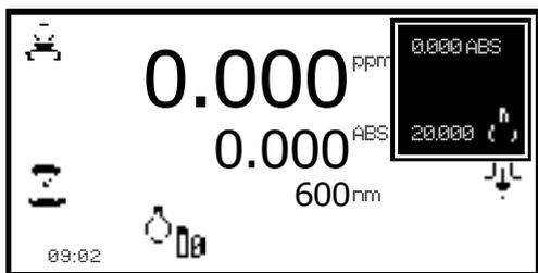
Press the key below the **calibrate to zero absorbance or standard** icon, this will open another menu with the option to re-calibrate to zero absorbance or to calibrate to the previously entered standard value. Press the key adjacent to the **calibrate to standard** icon.
