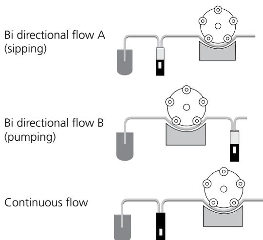
The tubing should be connected depending on the function that the sipper pump is going to perform. All tubing must be kept as short as possible and the tubing must not be allowed to obstruct the light path.
