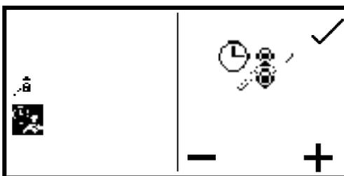
To fine tune the amount of sample uptake press the key below the **plus** or **minus** icon to increase or decrease the amount of sample taken up. The recorded time will be adjusted accordingly. Once the fine tuning is complete, or if none is required, press the key adjacent to the **tick** icon to move to the next stage of the calibration sequence.
