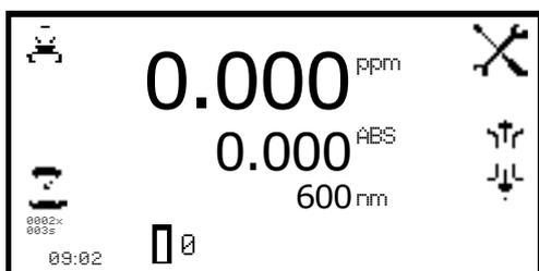
In the concentration measurement mode calibrations against a standard or a factor can be performed following a zero calibration. If the factor is not known calibration against a known standard is performed in order to calculate the factor. However if the factor is known there is no need to calibrate using a standard. The calibration must be performed at the same wavelength at which the sample will be measured.
