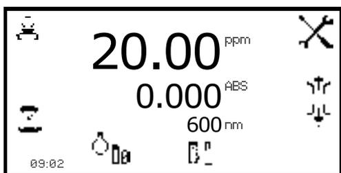
The instrument will take a reading and calibrate to the standard concentration. Once the calibration is complete the sample can be measured using the **measure to standard** icon.
