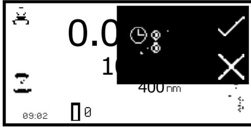
Confirmation will be needed to start the sipper pump. Press the key adjacent to the **cross** icon to cancel and return to the expanded operating menu. Press the key adjacent to the **tick** icon to confirm and start the sipper pump. The pump will run for the previously recorded air gap take up time.
