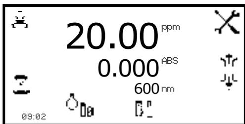
Remove the cuvette containing the standard sample and place a cuvette containing the sample to be measured in the sample chamber. Close the instrument lid and press the key below the **measure to standard** icon. Once the measurement is complete the concentration and absorbance values are displayed.
