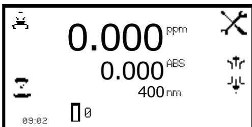
The wavelength can be adjusted in the expanded operating menu or in the settings menu. To adjust the wavelength in the expanded operating menu use the keys adjacent to the **arrow** icons to increase or decrease the wavelength.
