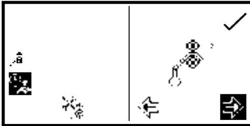
Press the key below the **calibrate timed sipper** icon. Select the required pump direction by pressing the key below the **forwards** or **backwards arrow** icon. Press the key adjacent to the **tick** icon to continue to the next stage of the calibration sequence.
