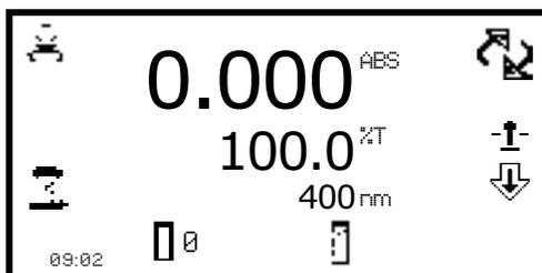
This measurement mode is very simple and the only parameters which can be adjusted are the wavelength and the display format.
