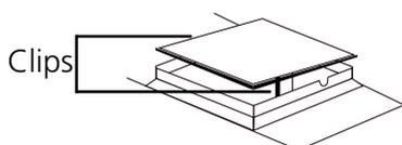
Use a small screw driver to lift the blanking panel on the top of the instrument. Squeeze the two clips in order to remove the blanking panel. Disconnect the printer wires which are secured to the underside of the blanking plate.
