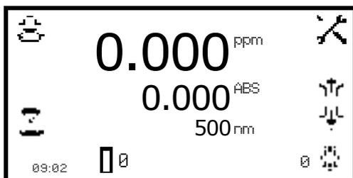
When the automatic 8 cell turret is in use the **8 cell turret** icon is displayed in the bottom right hand corner of the screen. The current cell position is displayed adjacent to the 8 cell turret icon. The 0 position should always be used for the zero calibration sample.
