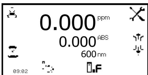
Insert a cuvette containing the blank solution into the sample chamber and close the instrument lid. Press the key below the **calibrate to zero absorbance** icon. The instrument will calibrate to zero absorbance. Once the calibration is complete the sample can be measured using the **measure to factor** icon.
