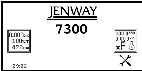
The time and date menu enables the current time and date to be set. This information will be saved on all results and displayed on printouts. The time and date menu can be accessed from the main menu by holding the key below the **time and date** icon for 2 seconds. Pressing the key once cycles the display between time and date.
