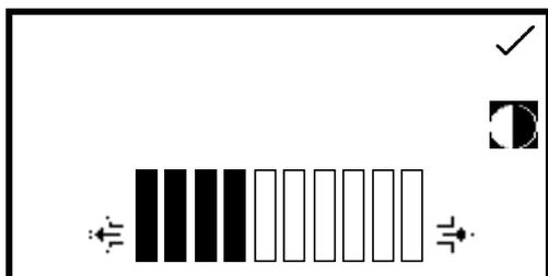
The screen contrast function enables the brightness of the screen to be set. In the instrument settings menu press the key adjacent to the **screen contrast** icon. Use the keys below the **arrow** icons to increase or decrease the screen contrast. Once the required contrast level has been reached press the key adjacent to the **tick** icon to save and return to the instrument settings menu.
