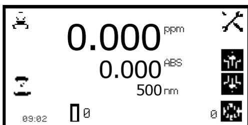
Press the key below the **8 cell turret** icon to highlight the icon and the two arrow icons above. Press the keys adjacent to the **arrow** icons to increase or decrease the current cell position of the turret, until the required sample position has been selected. Press the key below the **measure sample** icon. The instrument will perform a reading and display the result on the screen.
