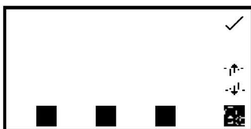
When this menu is first accessed the lamp save is turned off. To activate the lamp save function press the key below the **lamp save** icon. To deactivate the lamp save function press the key below the **lamp save** icon.
