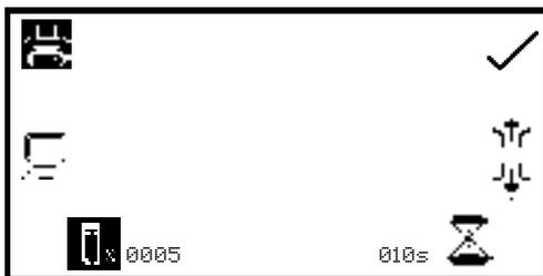
To set the time period between each measurement press the key below the **timer** icon and use the keys adjacent to the **arrow** icons to increase or decrease the time in 1 second intervals. To reset the time to one second press and hold the key below the **timer** icon for 2 seconds.
