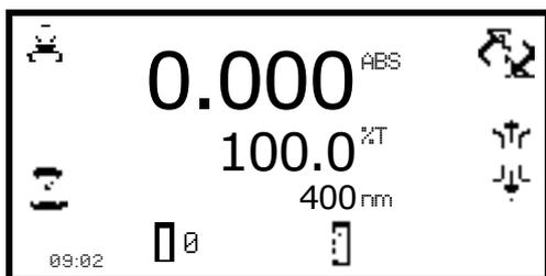
The calibration must be performed at the same wavelength at which the sample will be measured. Insert a cuvette containing the blank solution into the sample chamber and close the instrument lid. Press the key below the **calibrate to zero absorbance** icon. This sets the instrument to zero absorbance and 100% transmittance.
