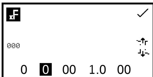
The factor menu enables a factor to be entered. This function is accessed by pressing the key adjacent to the **factor** icon. This opens the extended number entry screen. Use the keys at the bottom of the screen to select the digit to be changed. The key below the digit must be pressed twice to select the adjacent digit. For example 00 the first press of the key alters 10, the second press alters 01.
