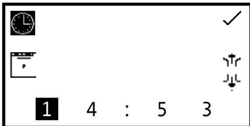
In the time and date menu to set the time press the key adjacent to the **clock** icon. Select the digit to be changed using the keys at the bottom of the screen. Use the keys adjacent to the **arrow** icons to increase or decrease the number. The clock function uses a 24 hour format.
