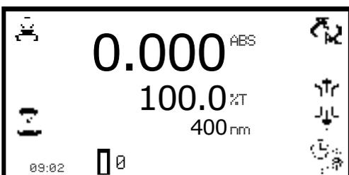
To perform a measurement place the sipper tubing into the sample and press the key below the **sipper pump** icon.
