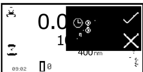
Confirmation will be needed to start the sipper pump. Press the key adjacent to the **cross** icon to cancel and return to the expanded operating menu. Press the key adjacent to the **tick** icon to confirm and start the sipper pump. The pump will run for the previously recorded sample take up time. Ensure that the flow through cuvette contains enough sample before pressing the key below the **measure sample** icon.
