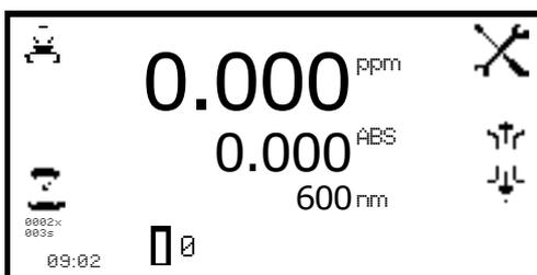
The number of repetitions and time period will be displayed below the autolog icon. To commence autologging press the key below the measure **sample** icon. Once the first measurement has been performed the time period starts counting down until it reaches zero and then the next measurement will be taken.
