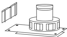
Take the 8 cell turret base plate. Connect the power supply in the bottom of the sample chamber to the connector on the underside of the baseplate. Place the base plate in the sample chamber. Replace screws 1 to 4.
