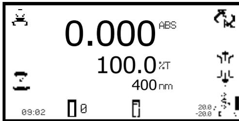
When the combined sipper peltier is in use the **sipper peltier** icon is displayed in the bottom right hand corner of the screen. The current temperature is displayed above the set point temperature adjacent to the sipper peltier icon. Adjacent to the peltier icon is an arrow to indicate if the current temperature is below or above the set temperature.
