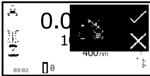
Once this stage of the calibration sequence is complete press the key below the **sipper pump** icon to dispose of the sample. Confirmation will be needed to start the sipper pump. Press the key adjacent to the **cross** icon to cancel and return to the expanded operating menu. Press the key adjacent to the **tick** icon to confirm and start the sipper pump. Depending on the disposal route previously selected the sample will either go to drain or back to the sample container.
