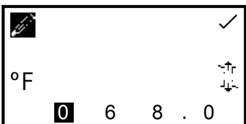
Once the required temperature has been selected press the key adjacent to the **tick** icon to save and return to the expanded operating menu. The peltier will begin to heat or cool depending on the current temperature.
