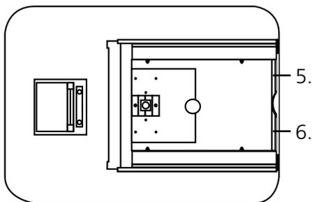
For this accessory as well as removing the passive accessory base plate, the front panel of the instrument must also be removed. Loosen screws 5 and 6 until the front panel can be lifted out in the forwards direction.
