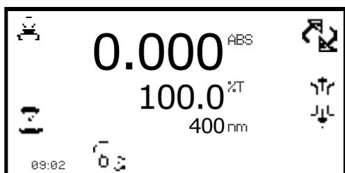
The time set will begin to count down when there is no lamp activity. When the count down is complete the lamp and the fan will be turned off and the **lamp save** icon is shown in all the measurement modes. To bring the instrument out of the lamp save in order to perform a measurement press the key below the **lamp save** icon.
