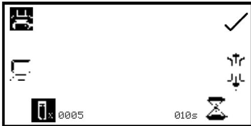
The autolog menu enables the result's destination to be set. To select the internal printer press the key adjacent to the **printer** icon. This option is only available if an internal printer is connected. To send the results to an external instrument such as a PC or a serial printer press the key adjacent to the **computer** icon.
