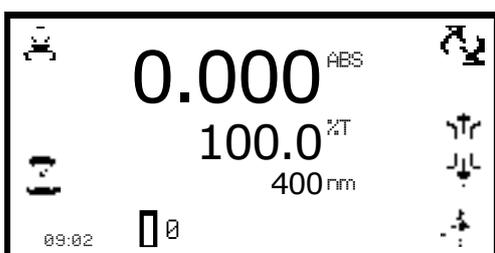
To perform a measurement place the sipper tubing into the sample and press the key below the **sipper pump** icon.
