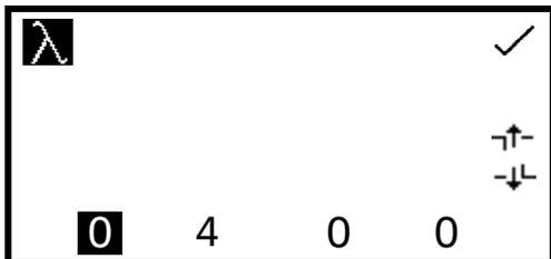
This will open a number entry screen. Use the keys at the bottom of the screen to select the digit to be adjusted. Use the keys adjacent to the **arrow** icons to increase or decrease the wavelength to the required number. Press the key adjacent to the **tick** icon to save the changes and return to the settings menu.
