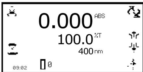
When the sipper is in use the **sipper pump** icon is displayed in the bottom right hand corner of the screen. The pump direction is displayed by an arrow icon below the sipper pump icon. The sipper pump can operate in manual or timed mode, depending on the option selected in sipper pump settings. To open the sipper pump settings hold the key below the **sipper pump** icon for 2 seconds.
