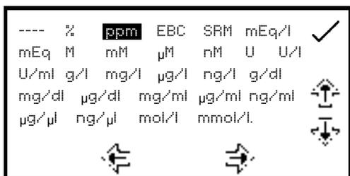
In the settings menu press the key below the **units** icon. This opens the unit selection screen which displays all the different units. Use the keys adjacent to the **arrow** icons to navigate around the screen to select the required units. Once the required units have been highlighted press the key adjacent to the **tick** icon to save and return to the settings menu. The selected unit will be displayed in the minimal and expanded operating menu along with absorbance and selected wavelength.
