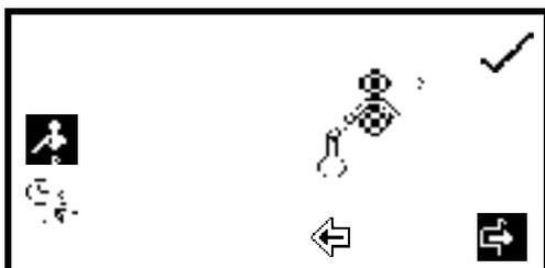
To operate the sipper pump in manual mode press the key adjacent to the **manual sipper** icon. Select the preferred pump direction by pressing the key below the **forwards** or **backwards arrow** icon. Press the key adjacent to the **tick** icon to save and return to the expanded operating menu.
