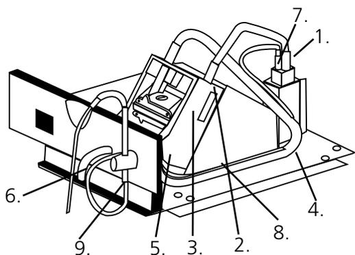
1. Connect the sipper pump tubing to the outlet port on the flow-through cuvette.
