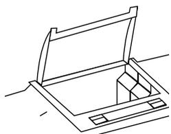
Squeeze the grey plastic clips together so that the printer top opens. Slot the printer into the top of the instrument and push down until it fits flush to all four sides.
