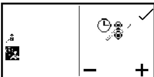
To fine tune the amount of air uptake press the keys below the **plus** or **minus** icons to increase or decrease the amount of air taken in. The recorded time will be adjusted accordingly. Once the fine tuning is complete, or if none is required, press the key adjacent to the **tick** icon to move to the next stage of the calibration sequence.
