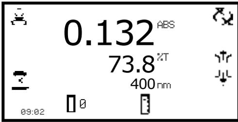
Results displayed in the expanded operating menu can be printed by pressing the key adjacent to the **printer** icon. Depending on the printout destination previously selected the result will be sent to the internal printer or the external printer. If the printer icon is pressed when there is not a result on the screen the **no result to printer** or **no result to RS232** icon (depending on results destination) will flash up on the screen.
