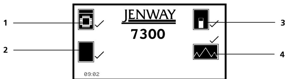
**Fig 2.2.2 – All Power On Tests Complete**
