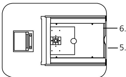
For this accessory as well as removing the passive accessory base plate, the front panel of the instrument must also be removed. Loosen screws 5 and 6 until the front panel can be lifted out in a forward direction.
