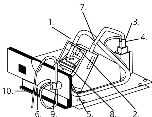
**1.** Cut two pieces of sipper pump tubing approximately 300mm in length. Take one length of tubing and fit this to the pump head, as shown, securing the tubing using the clip on the right hand side of the pump head.
