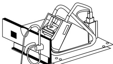
Take the sipper base plate. Connect the power supply in the bottom of the sample chamber to the connector on the underside of the base plate. Place the base plate in the sample chamber. Replace screws 1 to 4. Take the sipper front panel and slot into place before re-tightening screws 5 and 6.
