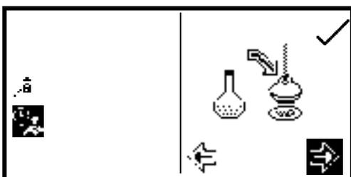
Once the sample uptake and air gap have been programmed the preferred disposal of the sample can be set. There are two options, the sample can either be sent back to the sample container or it can be sent to the waste pipe. Press the key below the **forward** or **backward arrows** to select what happens to the sample after measurement.
