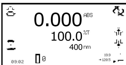
When the peltier is in use the **peltier** icon is displayed in the bottom right hand corner of the screen. The current temperature is displayed above the set point temperature adjacent to the peltier icon. Below the peltier icon there is an arrow icon to indicate if the current temperature is below or above the set temperature. To adjust the set point temperature hold the key below the **peltier** icon for 2 seconds.
