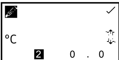
This opens the peltier settings screen. Use the keys at the bottom of the screen to select the digit to be changed and use the keys adjacent to the **arrow** icons to increase or decrease the number. The temperature can be set in °C or °F by pressing the key adjacent to the **°C** icon. Repeat presses will cycle between °C and °F.
