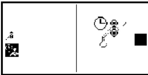
Once the cuvette is full press the key adjacent to the **stop** icon to stop the sipper pump. The time taken for sample uptake is recorded.
