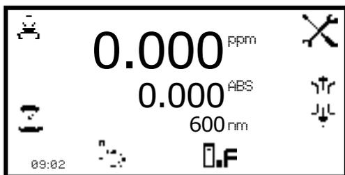
Remove the cuvette containing the blank solution and place a cuvette containing the sample to be measured in the sample chamber. Close the instrument lid and press the key below the **measure to factor** icon. Once the measurement is complete the concentration and absorbance values are displayed.
