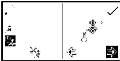
The settings menu is the same as the sipper pump settings except for the peltier icon in the top left hand corner. Pressing the key adjacent to the **peltier** icon will open the peltier settings enabling the temperature to be set. Refer to section 8.3.2 for more details. The sipper pump can operate in a manual or timed mode. Refer to section 8.3.3 for more details.
