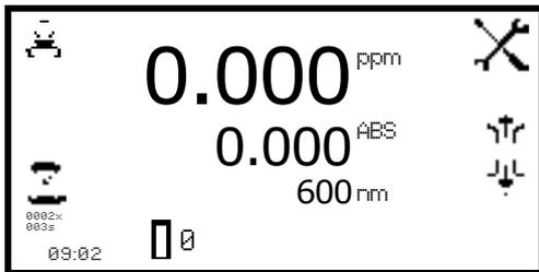
To open the print setup menu hold the key adjacent to the **printer** icon for 2 seconds in the expanded operating menu.
