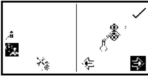
To operate the sipper pump in timed mode press the key adjacent to the **timed sipper pump** icon.
