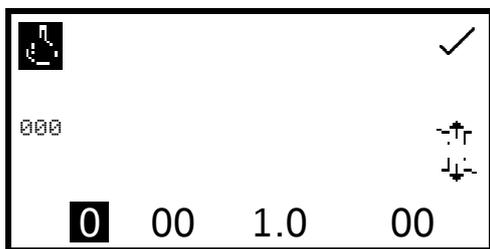
The standard menu enables the value of a standard to be entered. This function is accessed by pressing the key adjacent to the **standard** icon. This opens the extended number entry screen. Use the keys at the bottom of the screen to select the digit to be changed. The key below the digit must be pressed twice to select the adjacent digit. For example 00 the first press of the key alters 10, the second press alters 01.
