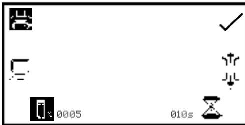
To set the number of repeat measurements of the same sample press the key below the **sample** icon and use the keys adjacent to the **arrow** icons to increase or decrease the number of repetitions required. To reset the number to zero press and hold the key below the **sample** icon for 2 seconds.
