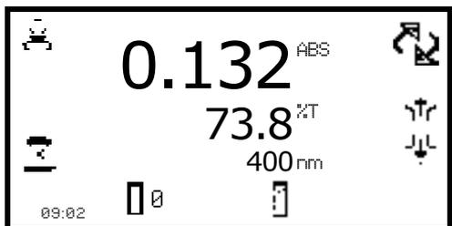
It is not possible to measure a sample before the instrument has been calibrated at the selected wavelength. Once the calibration has been performed the **measure sample** icon is displayed and a sample can be measured. Remove the cuvette containing the blank solution and place a cuvette containing the sample to be measured in the sample holder. Close the instrument lid and press the key
