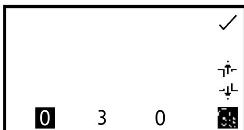
The default minimum time is set to 30 minutes. Select the digit to be changed using the keys at the bottom of the screen. Use the keys adjacent to the **arrow** icons to increase or decrease the number. Once the required time in minutes has been set press the key adjacent to the **tick** icon to save and return to the instrument settings menu.
